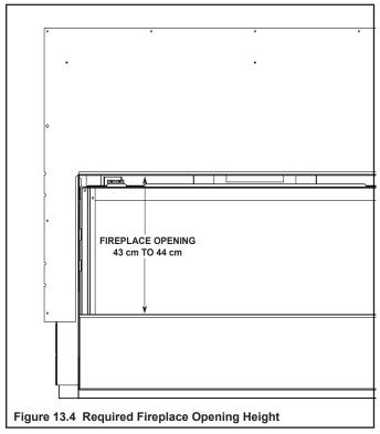
**Note:** The lower cover panel must be pushed all the way down. The outer finishing flanges should line up. The fireplace opening must be between 43 cm and 44 cm for the decorative fronts to fit correctly. See Figure 13.4.
